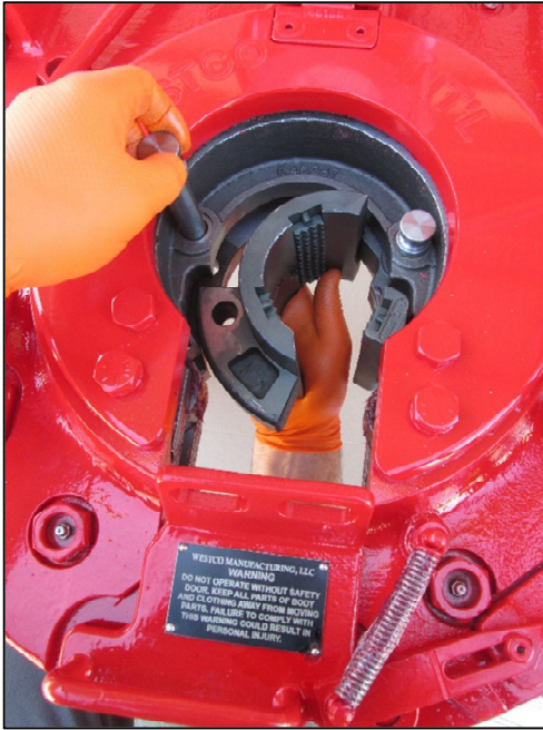
Figure 3: Installation/removal of bushing
