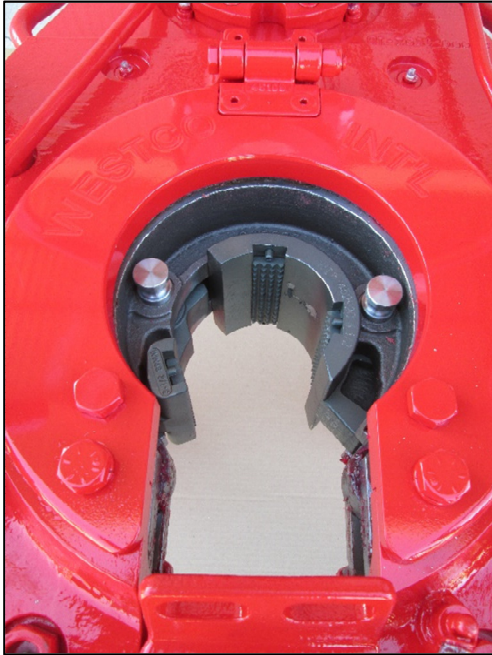
Figure 1: Jaws Installed (Break-out)
