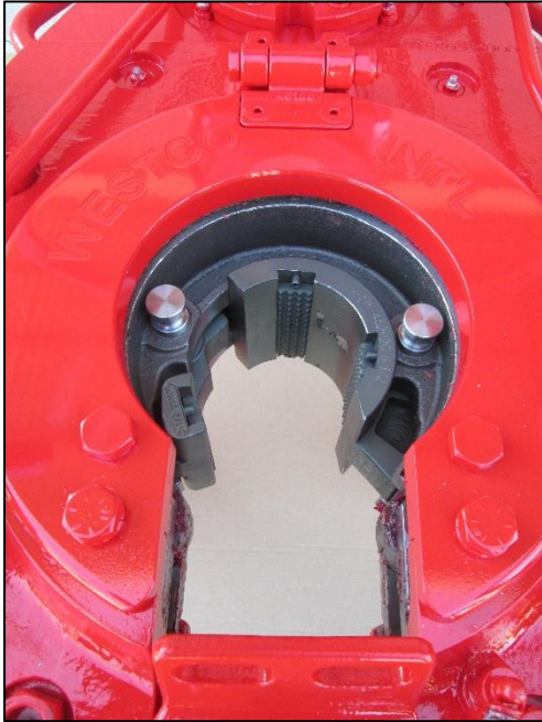
Figure 1: Jaws Installed (Break-out)
