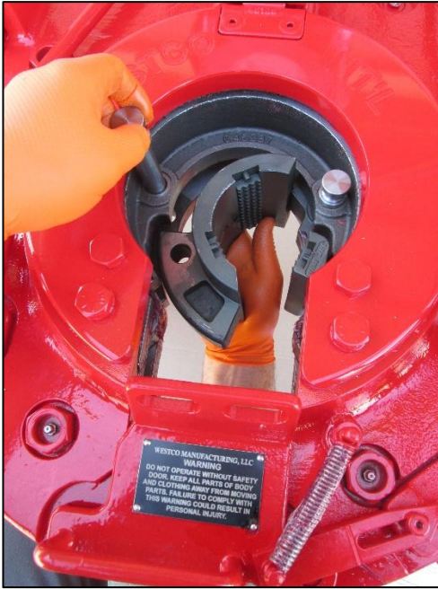
Figure 3: Installation/removal of bushing
