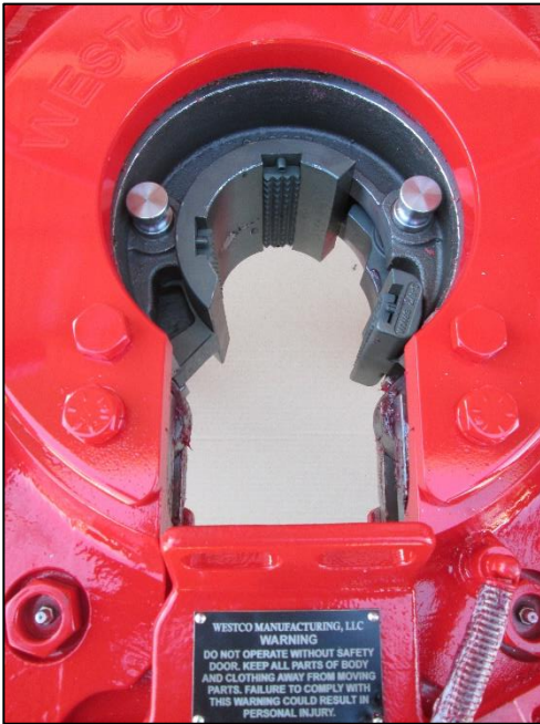
Figure 2: Jaws Installed (Make-up)
