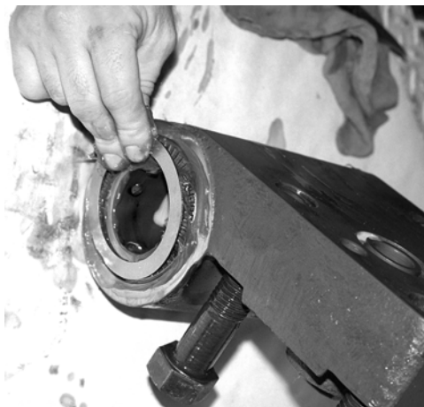
Figure 4-10. Installing Bracket Bearing
