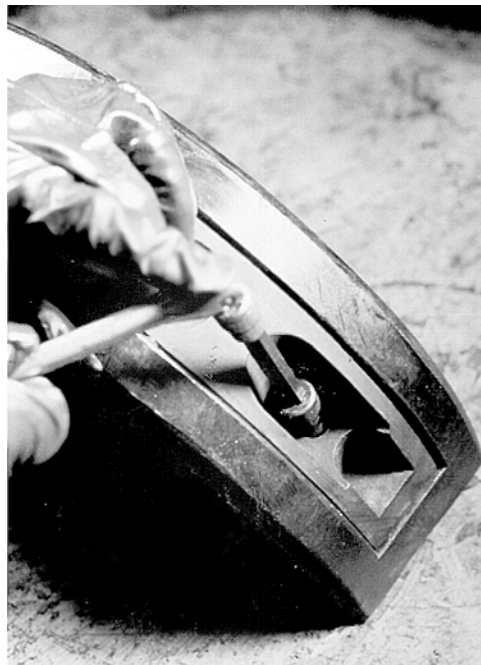
Figure 4-15. Removing the Ram Rubber Retaining Screws
