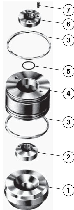
Figure 5-10. Manual Lock Piston Assembly
