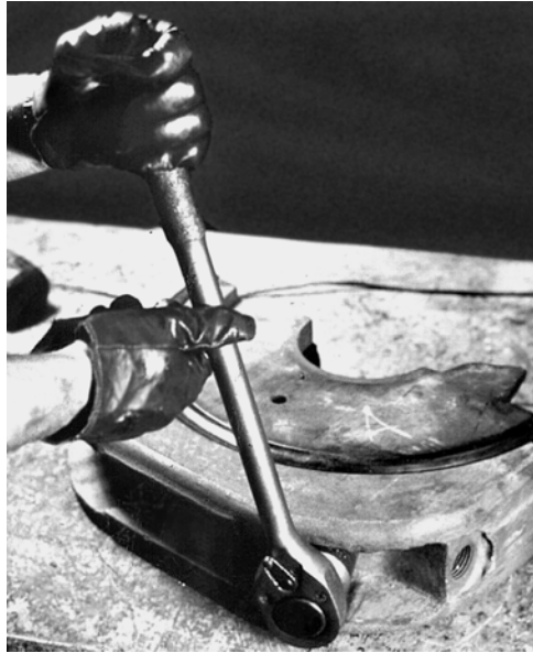
Figure 4-14. Removing the Ram Block Retracting Screws
