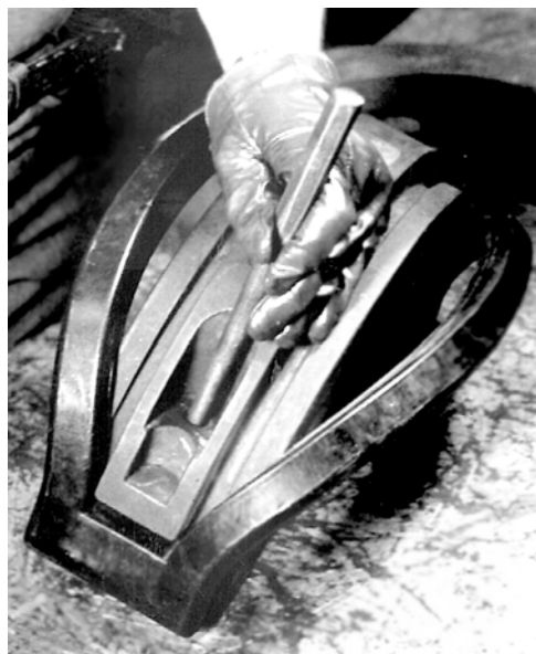
Figure 4-17. Driving the Ram Rubber out of the Block
