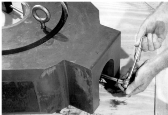
Figure 4-19. Remove Retainer Screw
