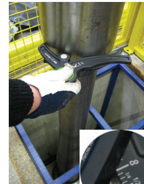
Measure pipe TJ-Diameter (OD) with 3-point measurement. Readout 8". The tool joint matches with the bore.
