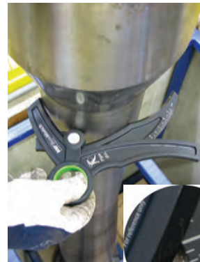
Measure pipe body (OD) with 3-point measurement. Readout 6". The pipe matches with the bore.
