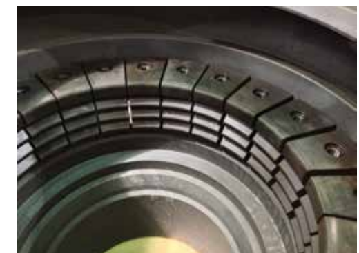
Locking Segment Coverage Shown in Unlocked Position
