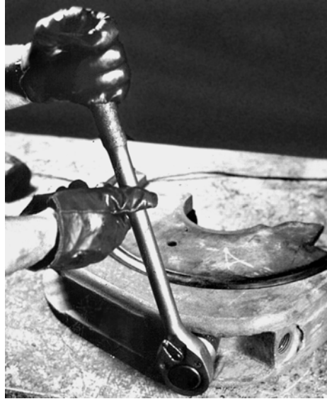
Figure 4-20. Remove Retracting Screws
