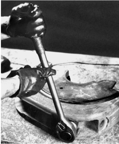
Figure 4-25. Install Retracting Screws
