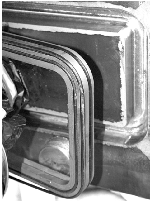
Figure 4-4. Remove Door Cartridge Seal
