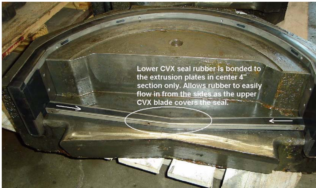
Figure 5-87. Lower Packer Bonding
