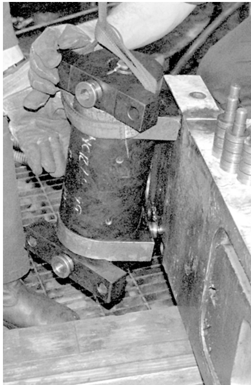
Figure 5-8. Lifting the Rotating Actuator
