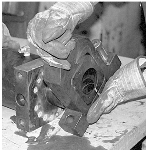
Figure 5-14. Removal of Rotary Actuator Idler Bracket
