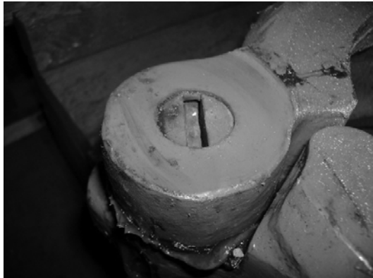
Figure 1: Lock bar removed correctly
