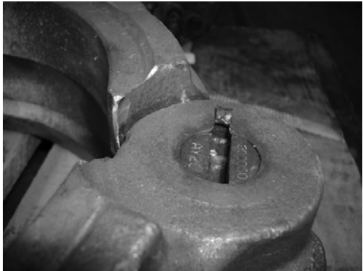
Figure 2: WRONG: Lock bar removed by driving shaft through from underside, causing damage to elevator.
