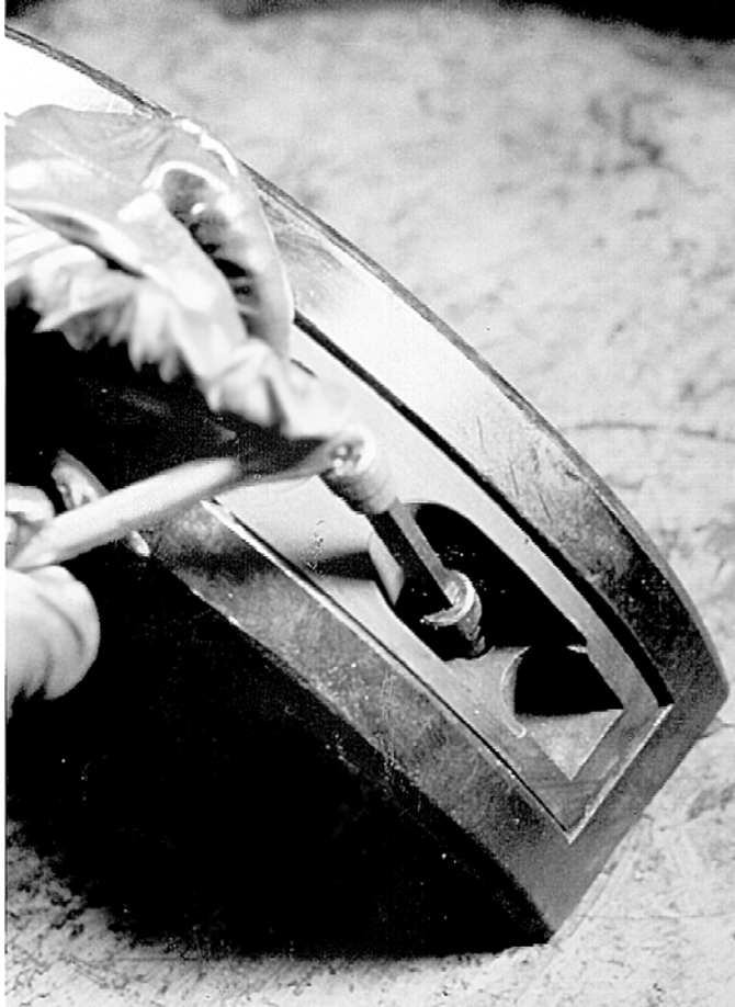
Figure 4-24. Install Retaining Screws
