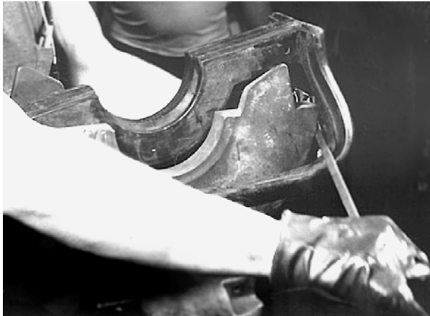
Figure 4-21. Install Ram Rubber
