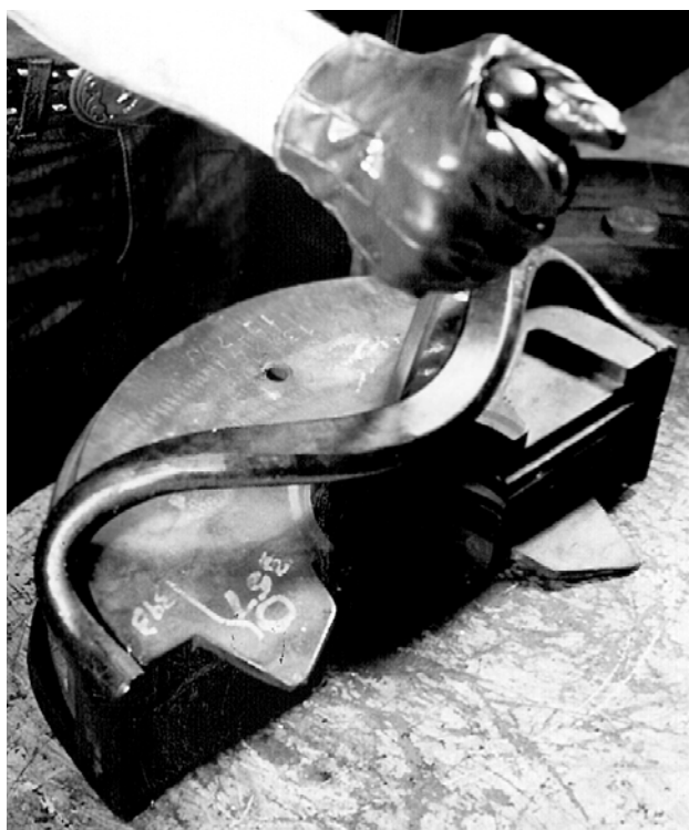
Figure 4-17. Pry Top Seal over Ram Block
