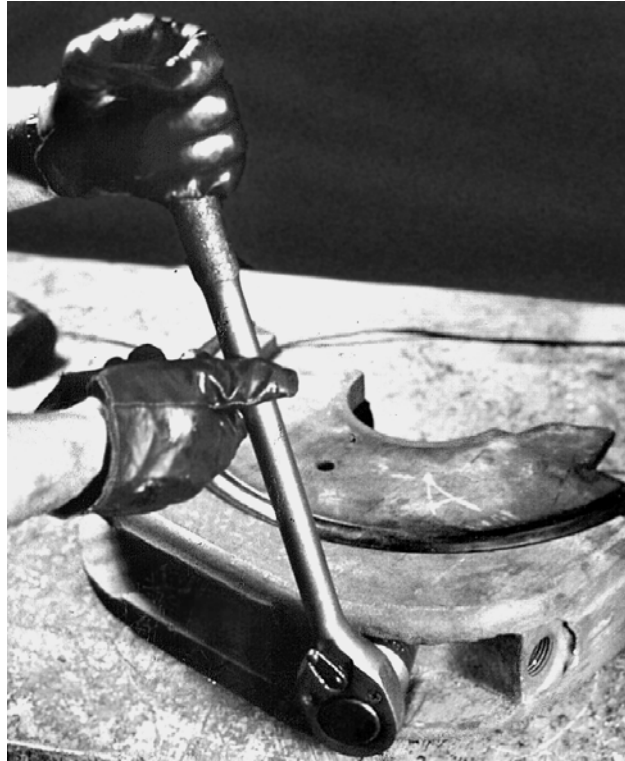
Figure 4-26. Install Retracting Screws
