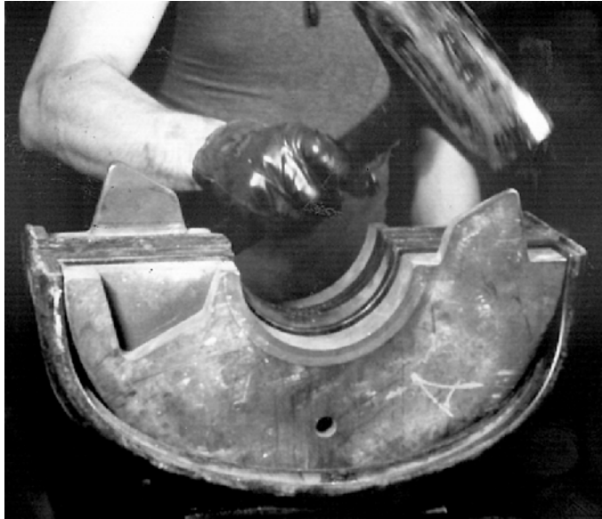
Figure 4-22. Hammer Ram Rubber into Ram Block
