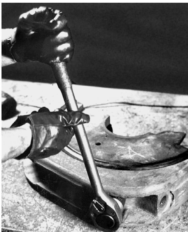
Figure 4-12. Remove Retracting Screws
