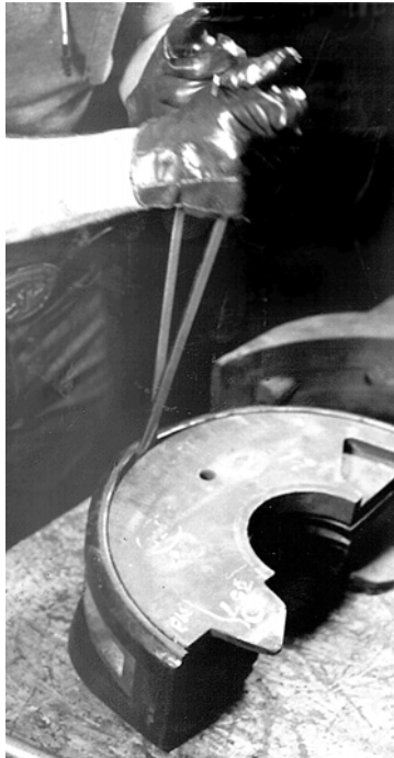
Figure 4-15. Insert Two Screwdrivers Between Ram Block and Ram Rubber
