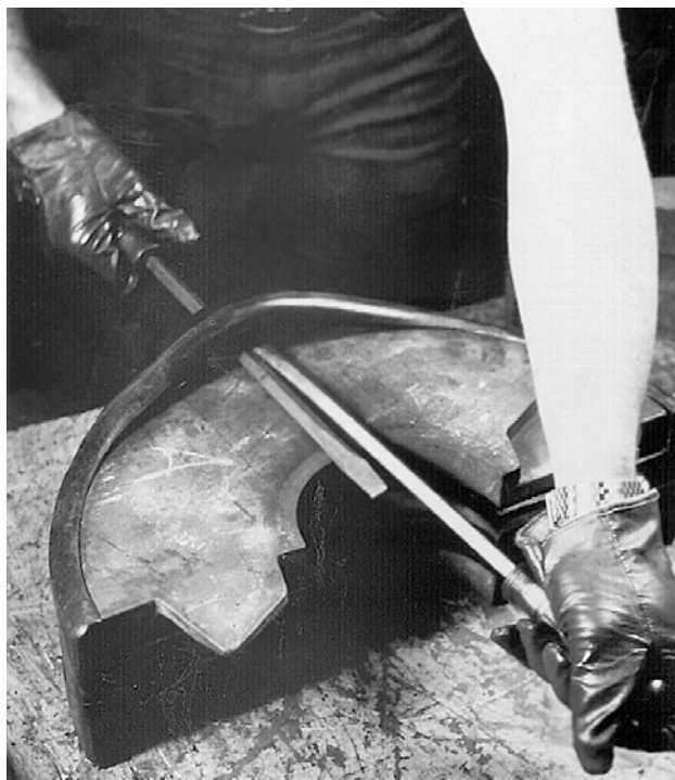
Figure 4-16. Pry Ram Rubber from Around Back Side
