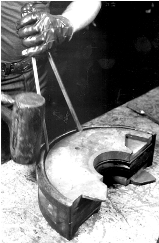
Figure 4-23. Pry Top Seal Over Ram Block
