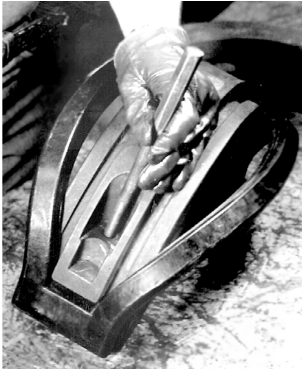
Figure 4-18. Use Punch to Remove Ram Rubber from Block
