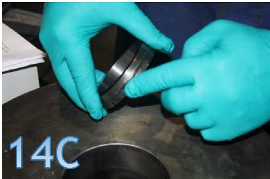
**14.** Check drive pin (picture 14A) to insure that it is not bent or missing, replace if required, Lube O-ring (Picture 14B) on stationary seal, line up notch to drive pin (Picture 14C) and install in stuffing box.
