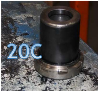
**20.** Slide mechanical seal onto sleeve (picture 20A), ensuring seal is at the back of the sleeve (picture 20B & C).
