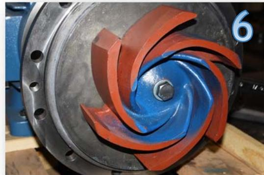
6. Using 1 1/8" deep socket, remove LEFT HAND threaded impeller bolt.
