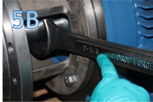
5. Secure main shaft on electric motor (Picture 5B) with 2 1/4" open end wrench.
