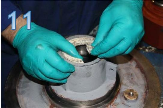
**11.** Remove rope packing and stationary seal assembly from stuffing box . (Picture 11).
