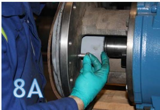
**9.** Remove shaft sleeve off motor shaft if still on, if problems occur with removal of the sleeve call Topco for assistance.
