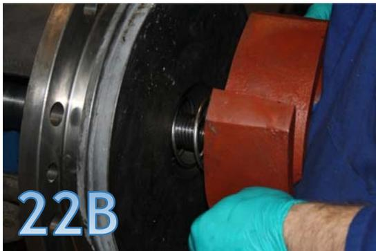
22. Place spring on back of impeller (Picture 22A), install impeller (Picture 22B).
