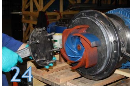
24. Using Topco Impeller Wrench (Part #79500) (Picture 24). Thread on (install) impeller in the clockwise direction.
