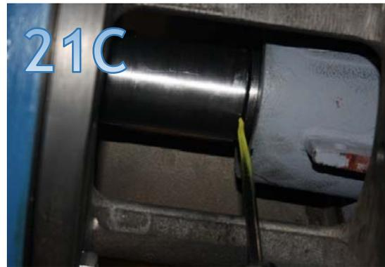
**21.** Install sleeve with mechanical seal face touching (Picture 21A) and push sleeve onto motor shaft (Picture 21B) until sleeve contacts O-ring. Ensure mechanical seal faces are seated (Picture 21C).
