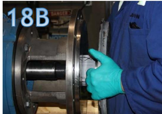
**18.** Install stuffing box onto C flange (Picture 18A) to the face (Picture 18B).
