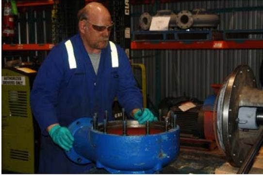
2. Use a 1 1/8" box wrench to remove nuts from pump housing.
